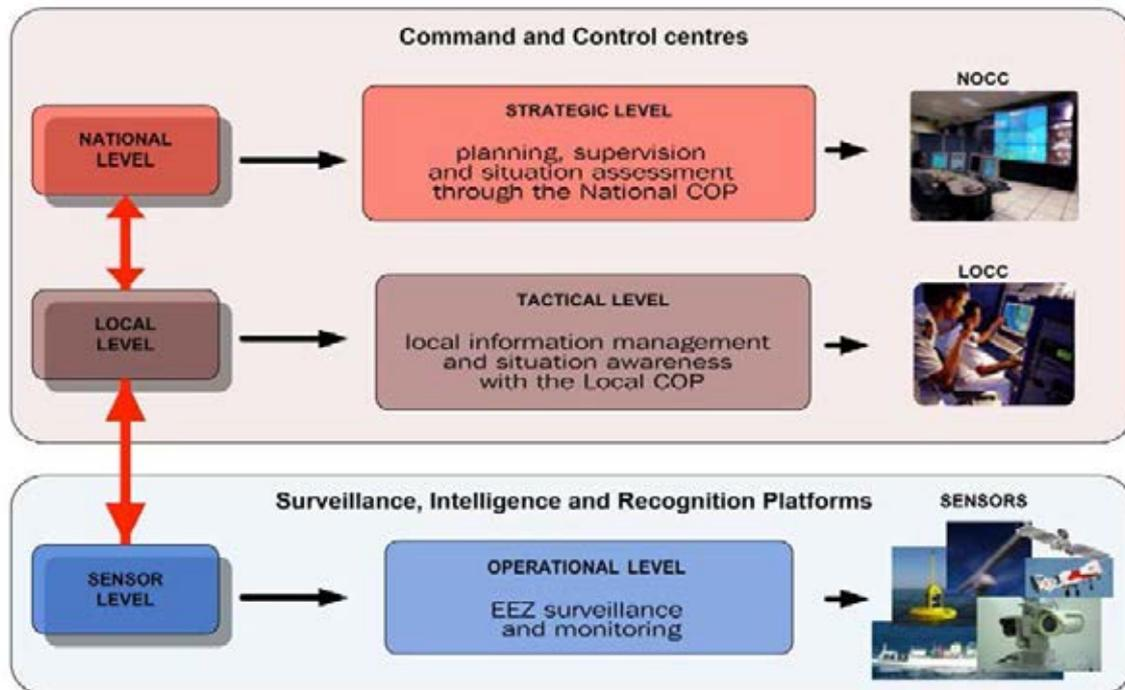
A solid net-centric communication and operational infrastructure connects and enables the integration of all subsystems and platforms that are part of the system architecture. The system consists of three different hierarchical levels.
