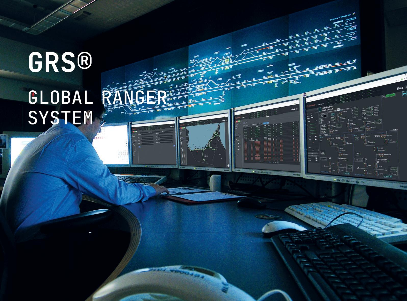
**Leonardo Global Ranger System (GRS®)** is a SCADA system to monitor and control heterogeneous remote processes or plants. It has been successfully used in several technology fields, such as energy transportation, oil & gas, energy distribution, electrical traction control and ancillary systems management.
